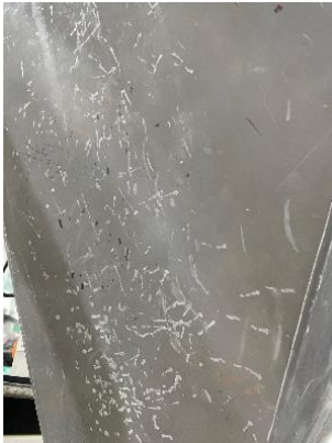
Figure 1: Effects of the hammer blows on the funnel (application A)
