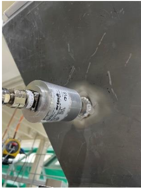
Figure 3: Ultrasonic converter on the aluminum hopper
