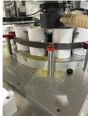
Figure 2: Improper dosing leads to product loss (application B)
