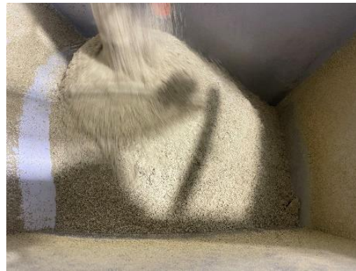
Figure 6: Smooth powder flow thanks to ultrasound
